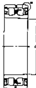
Tapered Bore MX-W222K Taper 1:12
